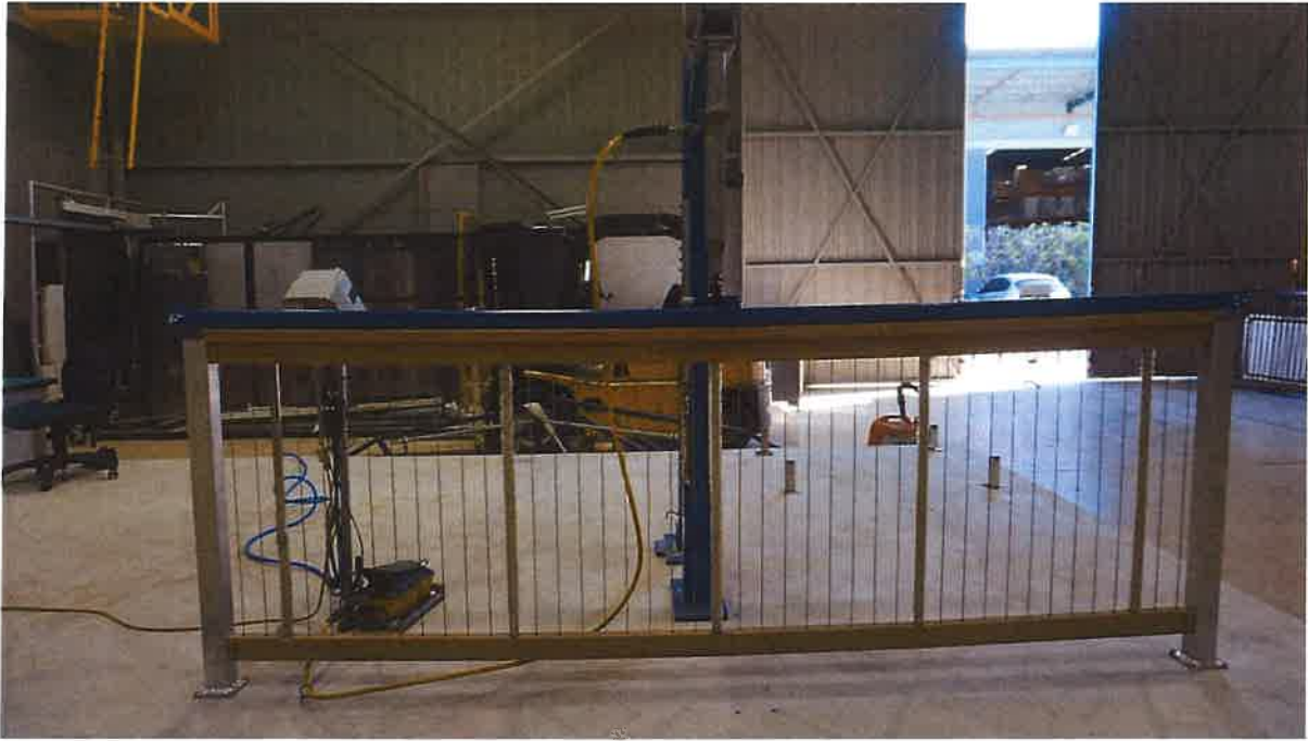
Figure 3: Vertical Uniform Ultimate Load
