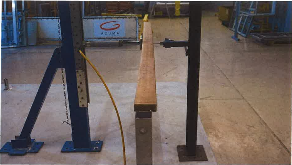
Figure 1: Outwards Ultimate Load
