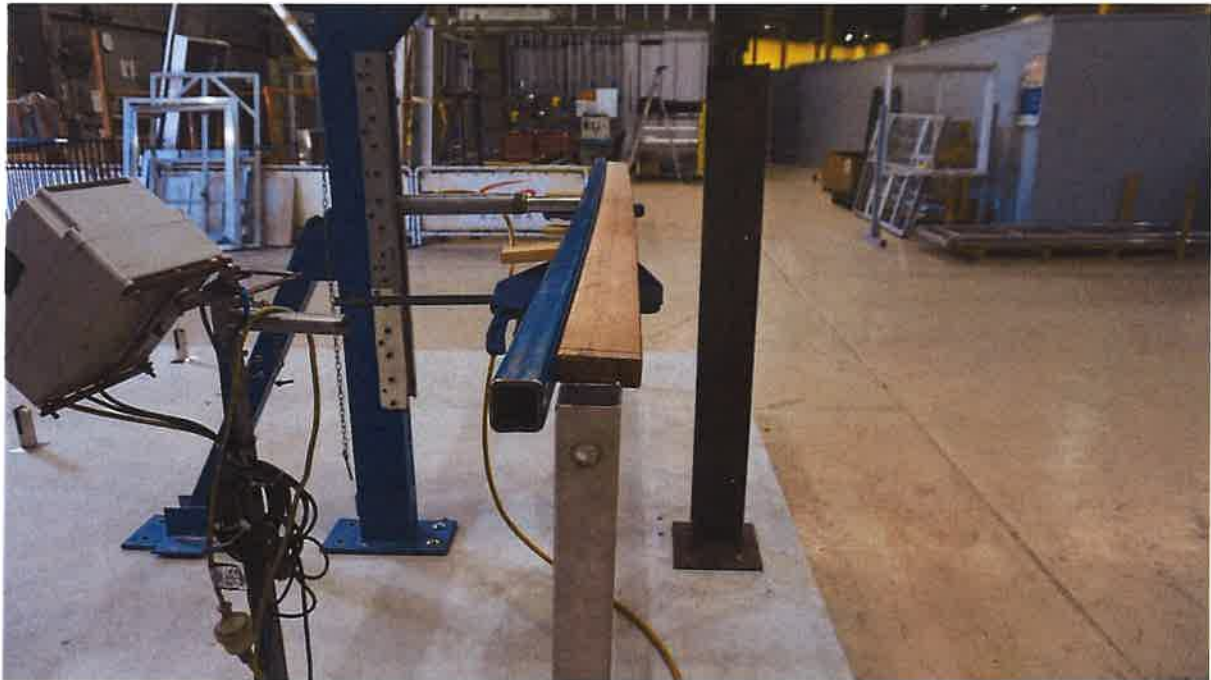
Figure 4: Horizontal Uniform Ultimate Load
