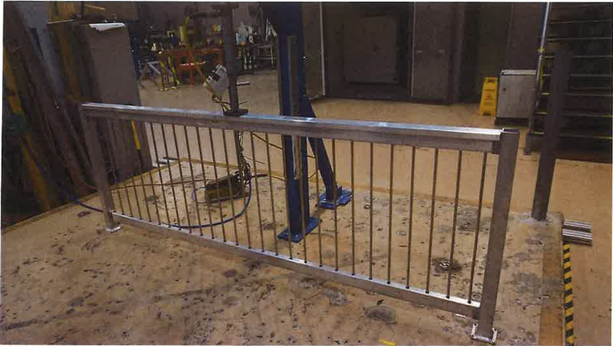
Figure 3: Serviceability Downwards Load
