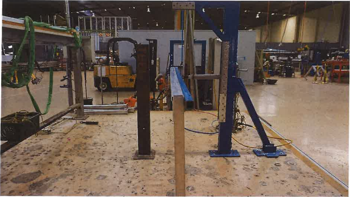
Figure 7: Serviceability Uniform Horizontal Load
