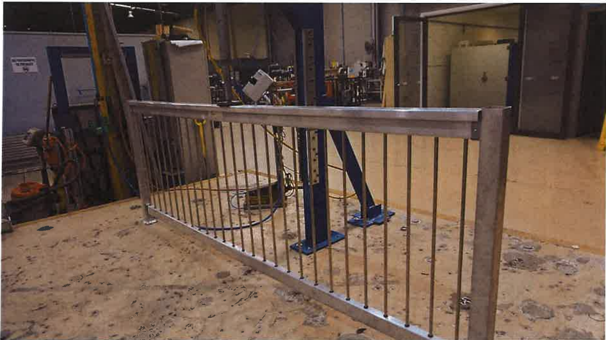
Figure 4: Ultimate Downwards Load
