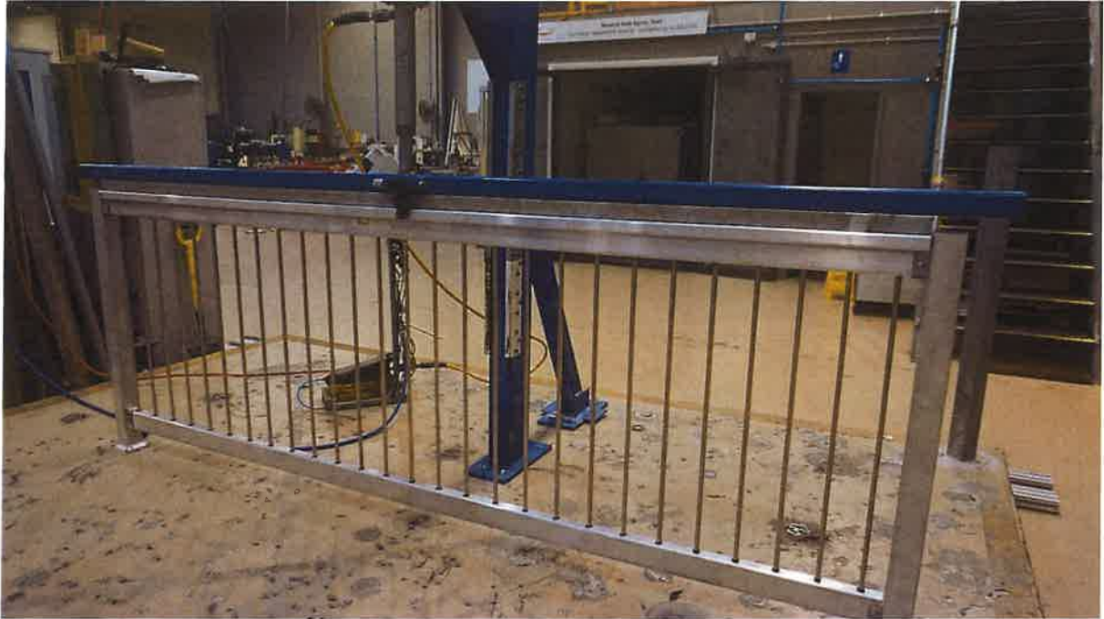
Figure 5: Serviceability Uniform Vertical Load
