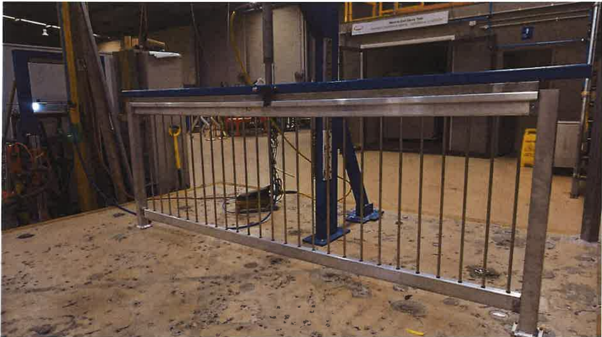
Figure 6: Ultimate Uniform Vertical Load
