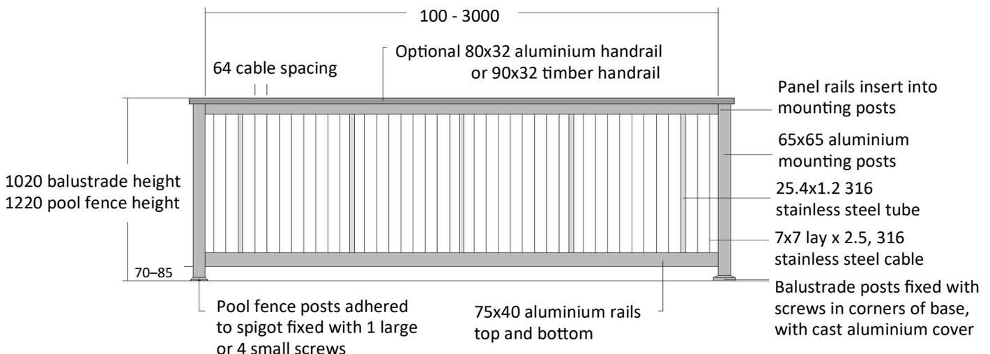
\* Rails over 2700mm must only be installed between existing, structurally sound posts
